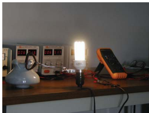
Figure 6. Compact fluorescent lamp running on DC power
