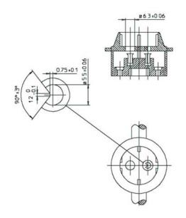
For other dimensions and specifications see standard sheet IV. The sketches are not intended to govern design except as regards the dimensions shown. Dimensions in mm.
