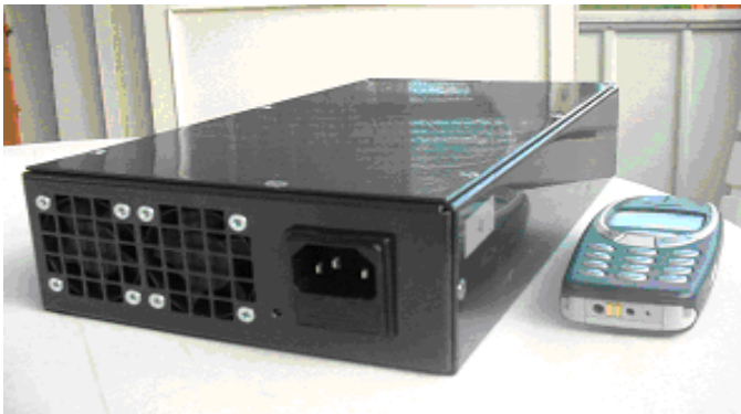
Fig. 2. 1.5 kW Rectifier – One of the key components of the HVDC system
