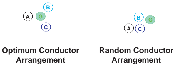
Induced ground currents come from asymmetry distribution of conductors within a conduit. This can be exacerbated by long cable runs.
